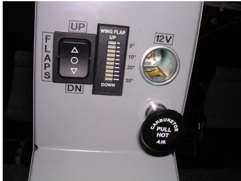
PICTURE 1 – LED Flaps position indicator
